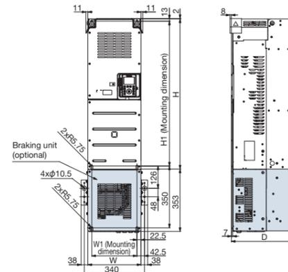
PB7-4200K is mechanically mounted on the left-hand side of the drive.
